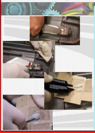
Mounting on an un-milled surface will cause a loss of some of the higher frequency signals, however it is sometimes the only choice:
