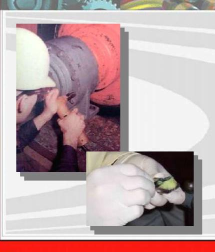
After an analyst decides which mounting hardware is best for the particular application, it is important that the proper technique for mounting the sensor and/or pad is used. Proper technique in mounting the hardware will ensure that the analyst is able to get the most out of the data collected.
